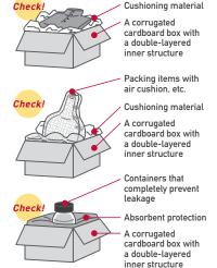
The box should be fastened securely in three places on both the top and
